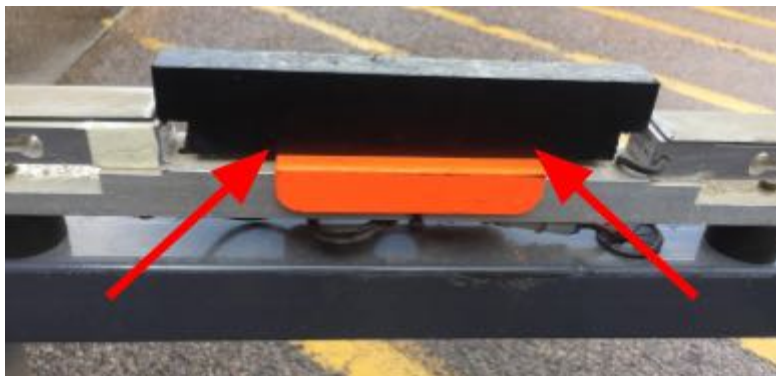
Figure 4) Load Cell Protection Spacers
