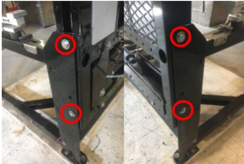
Figure 8) Loosen four bolts to raise/lower the front of SmartFeed
