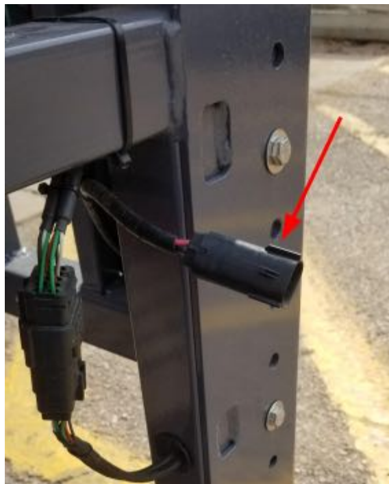
Figure 5) SmartFeed Power Receptacle
